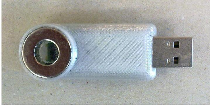
Figure 5: USB-IRDA configuration converter
