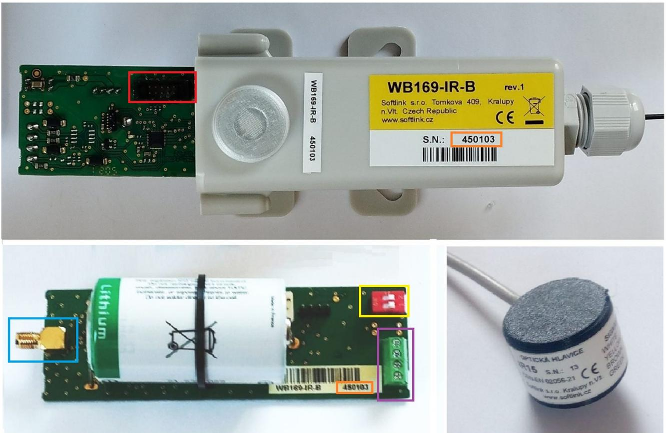
Figure 11: Detail of the printed circuit board of the WB169-IR-B module
