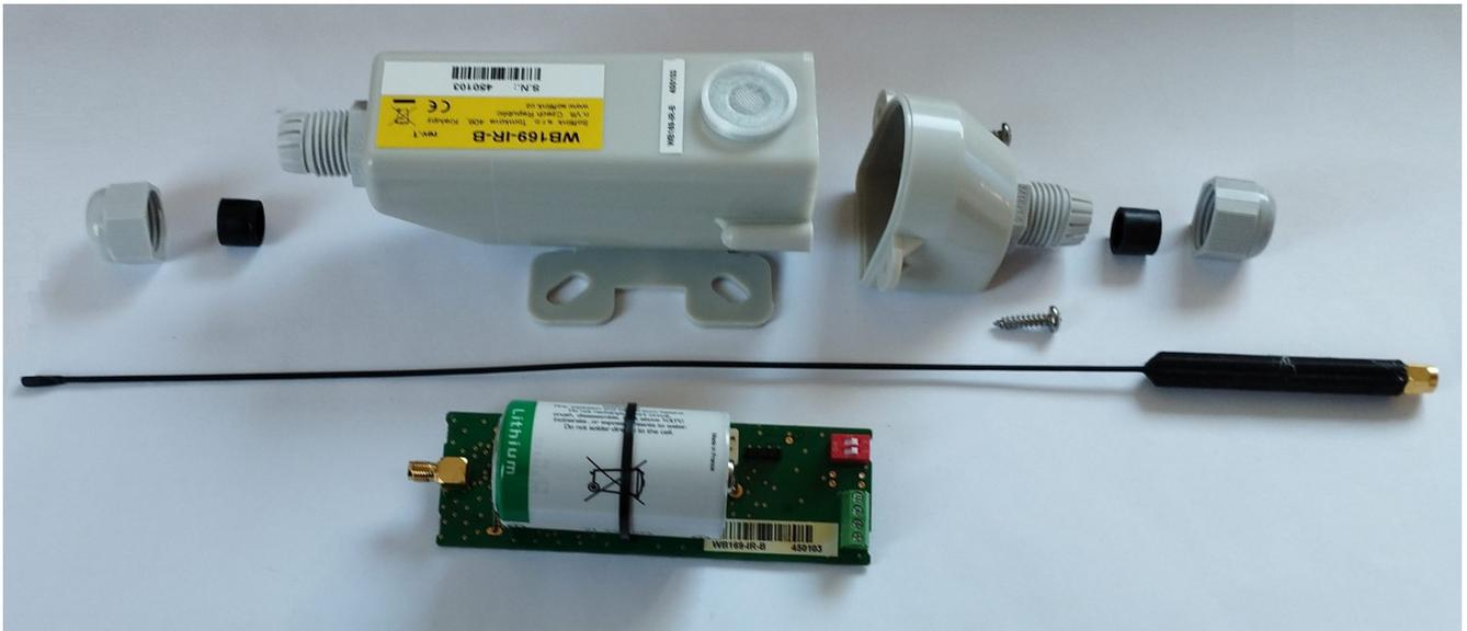
Figure 10: Assembly of the WB169-IR-B module with rod antenna
