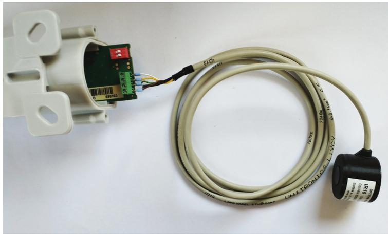
Figure 12: Connecting the optical head to the terminal block of the WB169-IR-B module
