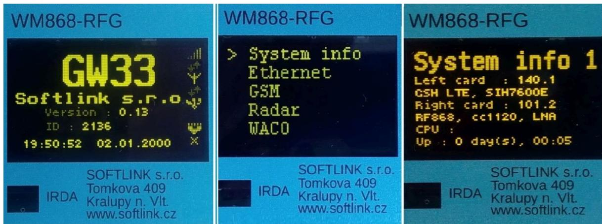
Figure 5: Display of the main screen, menu and system information
