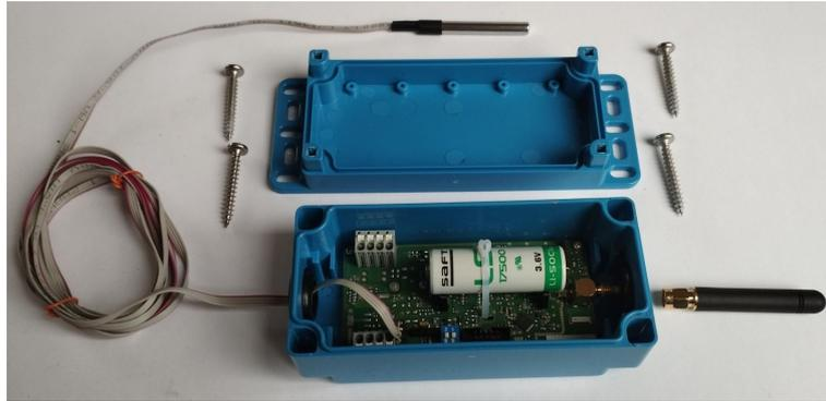
Figure 10: WM868-TE-B module assembly with rod antenna
