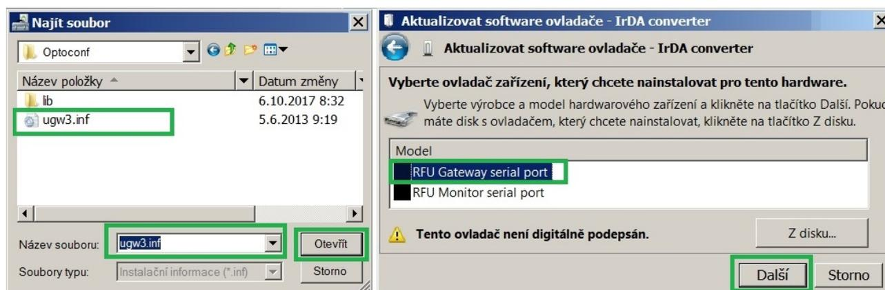
Obr. 9: Instalace driveru USB
